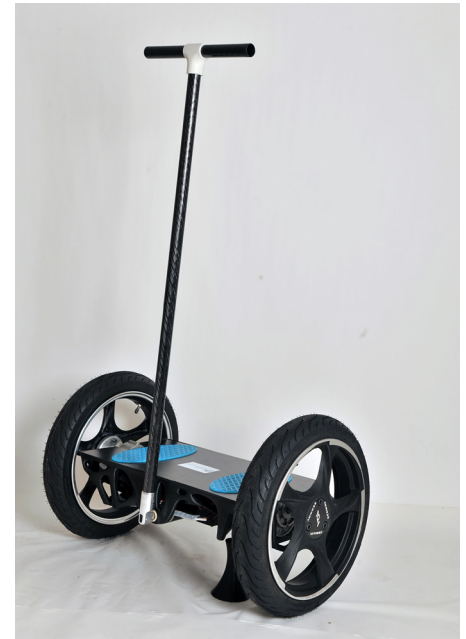
The finished self-balancing scooter designed and manufactured by the University of Applied Sciences Ravensburg-Weingarten.
